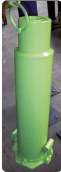
50 ton, 2 speed, long stroke bottle jack
