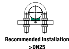
Round Steel U-Bolt (type RB) with Plastic Pipe Saddle (type RUK)
