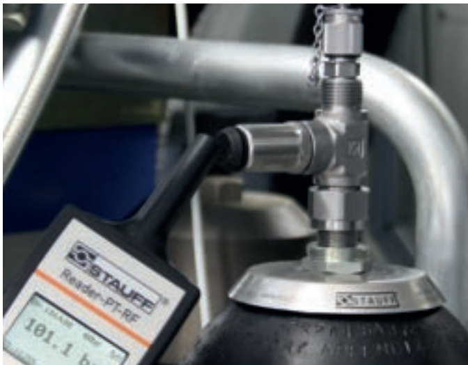
Bladder accumulator in use with Reader-PT-RF
